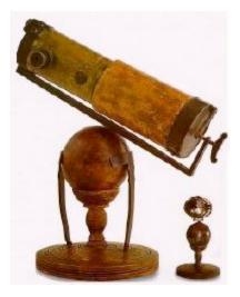
His selection of material to make the reflecting surface was an alloy of copper and tin. He polished and smoothed the mirror until he felt it overcame the aberrations caused by the refracting lenses. It actually took a while for his telescope to catch on but eventually as the technique was perfected the advantages of his design won over principally due to the much more manageable size and higher light gathering capability.
