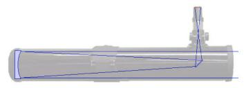
**Gregorian** – In 1663 a Scottish mathematician named James Gregory designed a telescope that had a small secondary mirror that reflected light through a hole drilled in the main mirror. The design also called for two concave mirrors, with the secondary mirror placed outside the focal point of the main mirror. Unfortunately, the technology of the mid-1600's could not produce mirrors accurate enough for his design to work properly.
