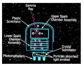
There are two types of Gamma-Ray detectors. The first are what would typically be called spectrometers or photometers in optical astronomy. These are instruments which are "light buckets" and focus on a region of the sky containing the object of interest collecting as many photons as possible... The second class is detectors that image gamma-ray emitions. Detectors of this type either rely on the nature of the gamma-ray interaction
